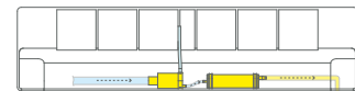
Water sensor and pump in the AC unit next to each other.
