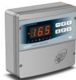
Fig. 3: Close the front panel, making sure that all the wires are inside the box and that the box seal sits in its seat properly. Tighten the front panel using the 4 screws, making sure the O-rings on the head of each screw are used. Give power supply to the panel and carry out a scrupulous reading / programming of all the parameters set.
