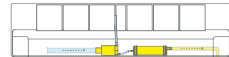
Water sensor and pump in the AC unit next to each other.
